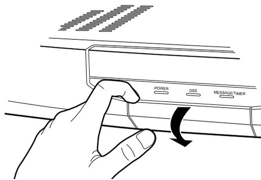
Then insert the card, arrow side up, as shown, and gently push the door up to close it.
